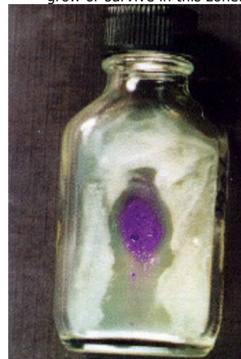
Note the fungus is unable to grow or survive within the clear area surrounding the Sav-A-Hoof Gel sample. Even with ideal growth conditions, with no oxygen and a growth medium, this area is fungus free and again represents the effective kill zone.
